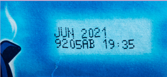
FIG 2. Typical low-resolution coding and marking print.
