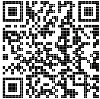
FIG 28: A QR Code using 2x2 pixels for each module.
